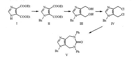
The reduction of diester II by lithium aluminum hydride in THF leads to 1-benzyl-4,5-di(hydroxymethyl)imidazole (III), the treatment of which with thionyl chloride gave dichloride IV. By cyclization of the latter with a disodium salt of diphenyl urea in dry DMFA, 1-benzyl-5,7-diphenylimidazo[4,5-e][1,3]diazepin-6-one (V) was isolated in a 20% yield. This low yield is most likely explainable by the possible intermolecular "crosslinks" of the starting dichloride IV and the urea used.
